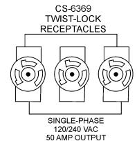
Figure 10. 120/240V Twist-Lock Auxiliary Receptacles
